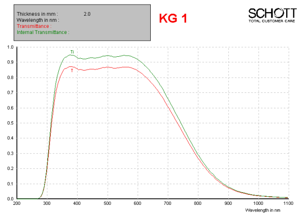
Figure 3.5: A graph to show the transmittance profile of a KG1 filter.
